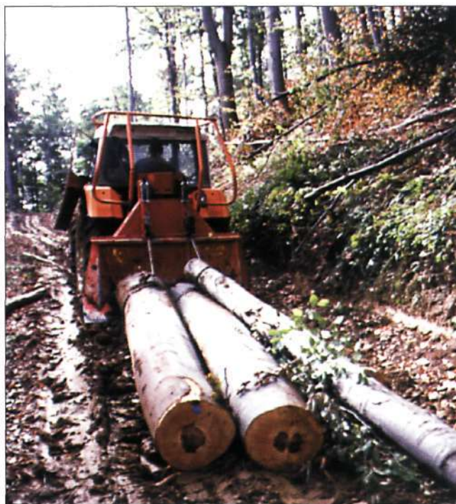
Slika 2. Traktor Steyr 9078 s vitlom Tajfun EGV 2 x 60 kN Figure 2 Steyr 9078 tractor with Tajfun EGV 2 x 60 kN winch
