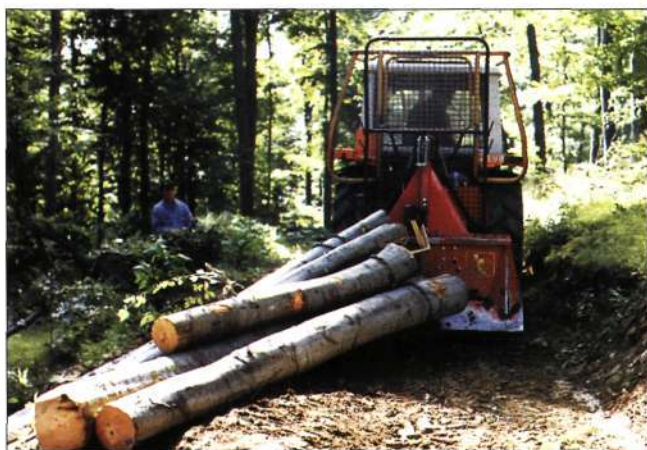
Slika 1. Traktor Steyr 8090 s vitlom Tajfun EGV 60 A Figure 1 Steyr 8090 tractor with Tajfun EGV 60 A winch
