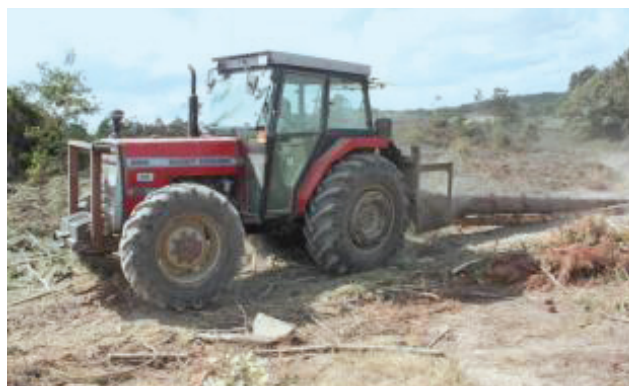
Figure 2. Timber skidding by farm tractor
